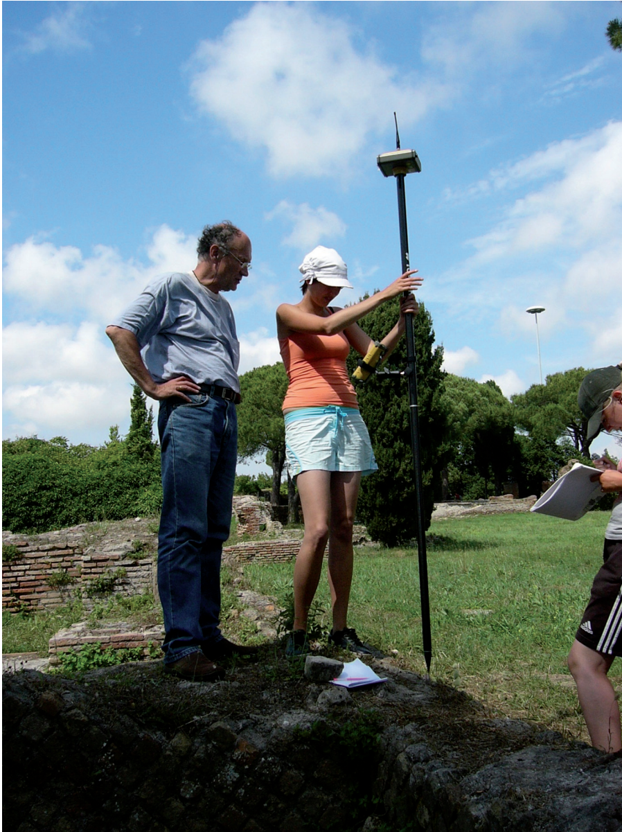
Figure 1. Differential GPS on reference points linked to architecture in Insula IV ii.
