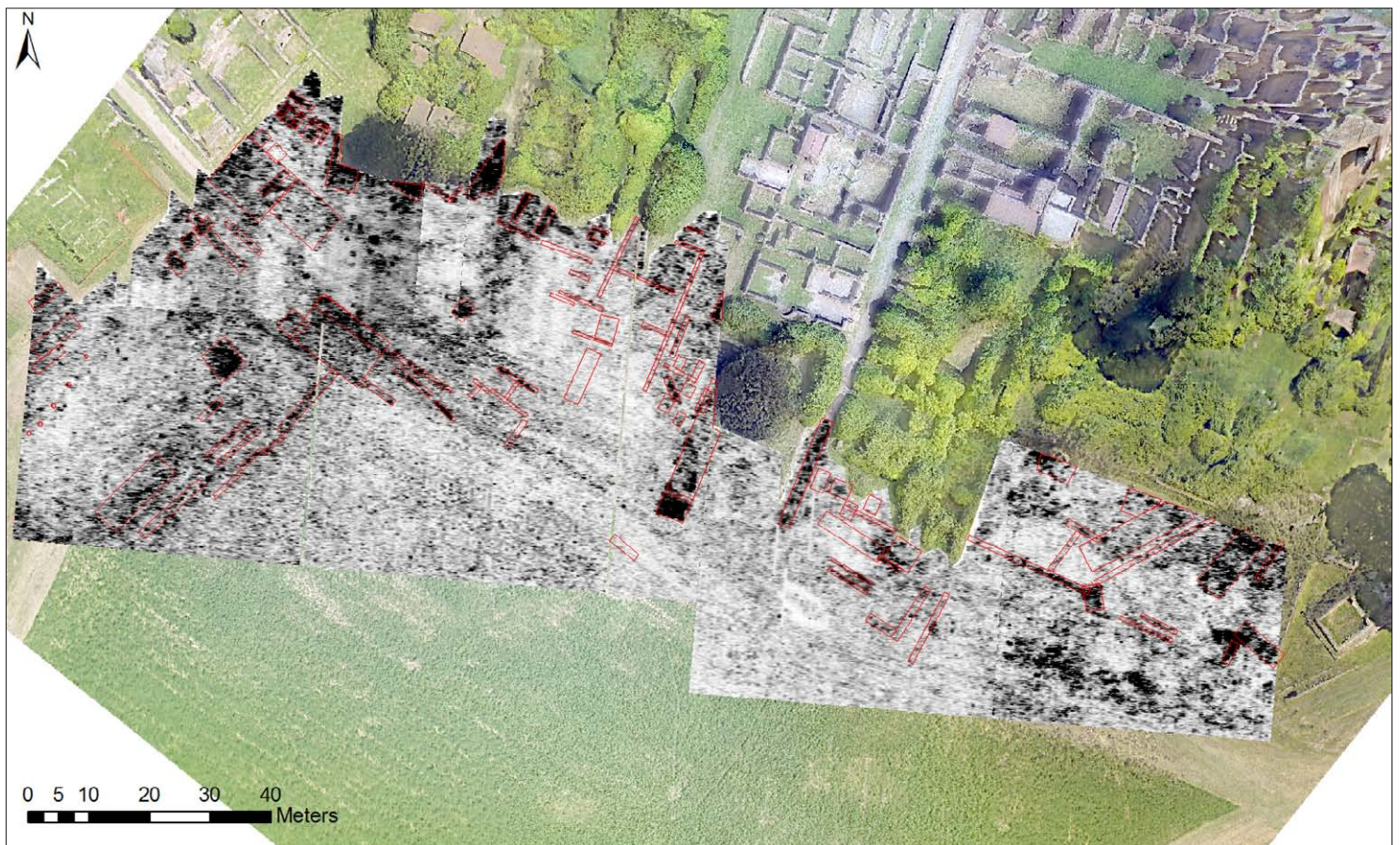
Figure 3 (below) GPR survey results (depth ~70-100cm), overlaying the UAS orthophotographs; highlighted in red are the structures identified so far.
