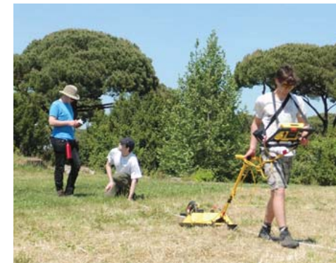
Fig. 4: Fieldschool 2015, Ostia, GPR survey, (students from Leiden, TU-Delft and Augsburg).
